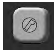
Unloading Auger Drive Engage/Disengage Switch and Indicator Light
