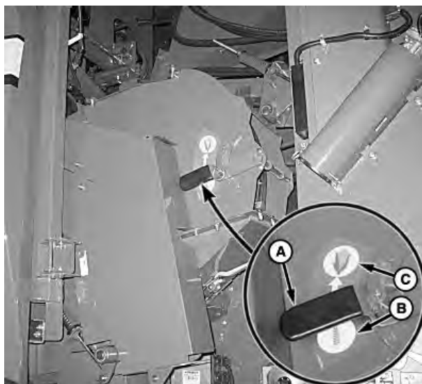
A—Crop Selection Handle B—Small Grain Position
